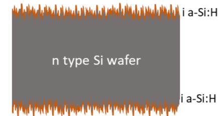
Figure 4. Cross-sectional view of passivation samples.
