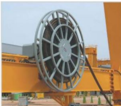
Cable reel for Big Crane
