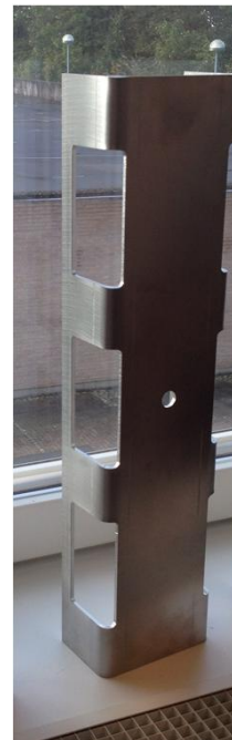
Embedded support prototype for Active Cell liner
