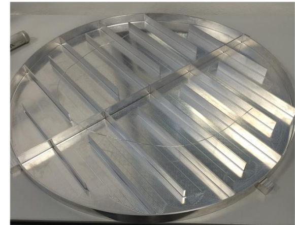
Prototype vessel for water pre-moderator (FZJ)
